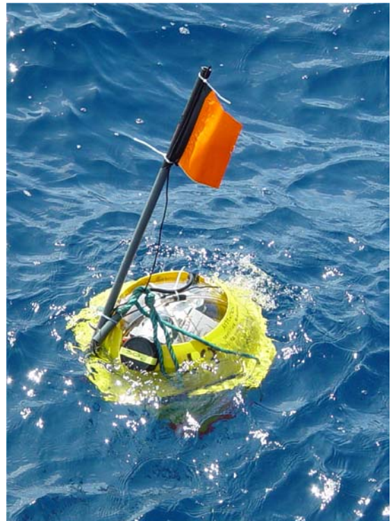
Figure 12: An OBS. All the OBS used were four component (three component seismometer and a hydrophone).
